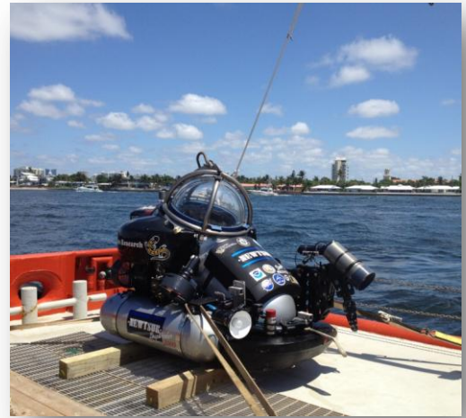
Loading the submersible onto the shipping vessel for transport to the habitat.
