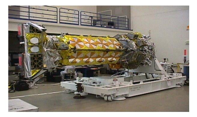
Figure 5-2: NOAA N Spacecraft in Horizontal Position on TOC
