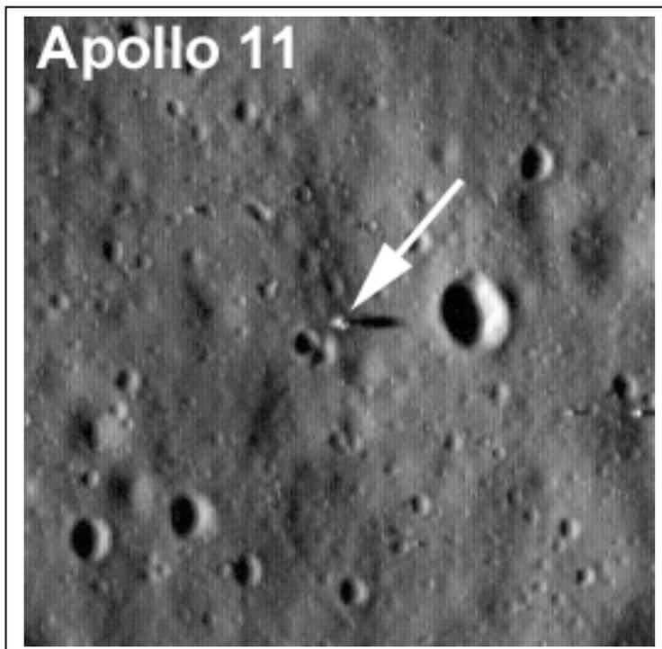
This LRO image was obtained in 2009 from an altitude of 60 kilometers above the Apollo-11 landing area. The **1-meter** resolution clearly shows the Apollo Landing Module that served as the launch pad for the returning Lunar Excursion Module (LEM) carrying Astronauts Armstrong and Aldrin.
