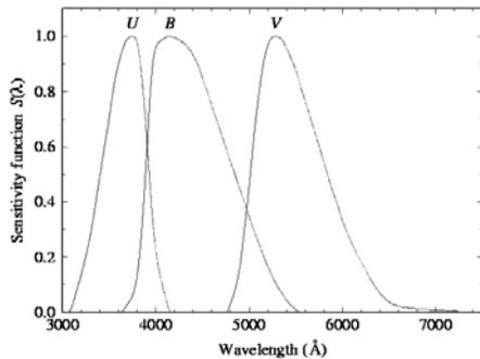
The 'UBV' set of filters are used in astronomy to classify the light from distant stars and galaxies. The U, B and V brightness of a star can be used to determine the star's temperature. For example, a hot star is brighter in the U-band than in the B or V bands. A cold star is brighter in the V-band than in the U or B bands.
