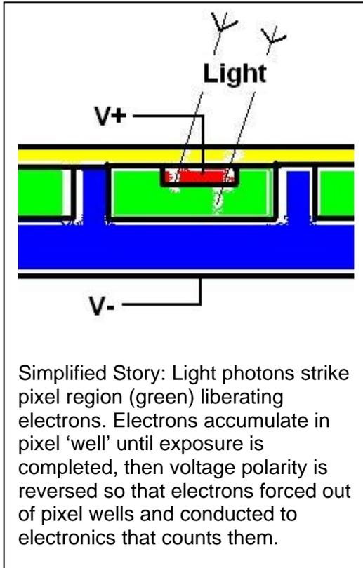
Each pixel in a CCD chip is a complicated electronic device called a photodiode. When a photon of light falls on the surface of the pixel, it interacts with the material in the pixel and causes an electron to be freed from its atomic 'prison'. This electron is then stored within the electronic components of the pixel.
