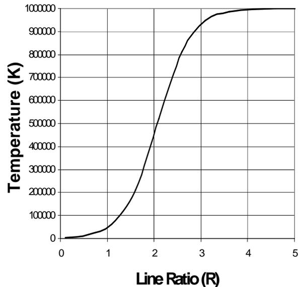
The light produced by heated gas is emitted in the specific spectral lines that the particular atoms and molecules are permitted to emit according to the rules of quantum mechanics. This also means that some specific lines can be used as a thermometer to determine the temperature of the gas they are a part of. Scientists can do this by selecting the specific atomic lines that work well as ‘thermometers’ and perform a simple calculation using the ratio of the line intensities.
