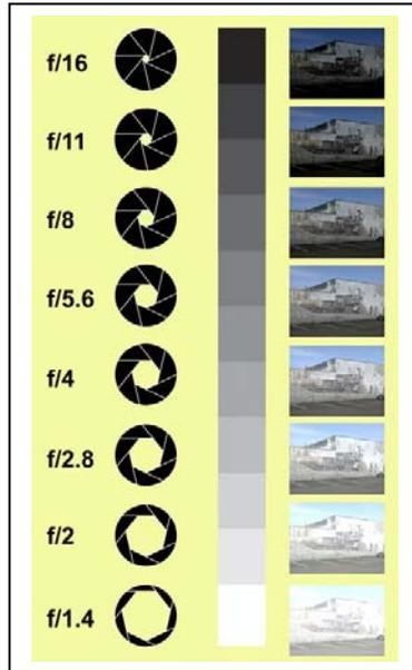
Digital cameras contain lenses that help gather photons into a concentrated beam. This beam comes to a focus on the CCD chip containing the pixels which detect the photons. The larger the area of the lens, the more photons can be collected.
