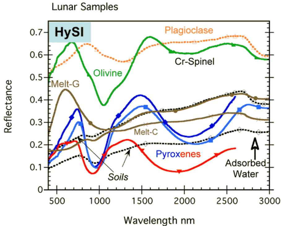
Lunar rock samples brought back by Apollo astronauts have been carefully examined, and represent many basic classes of minerals. The two most common are the pyroxene-A (blue line) and pyroxene-B (red line), which are found in the extensive lava fields of the lunar mare (dark areas), and plagioclase (orange line), which is found in the mountainous lunar highlands. The above graph shows the reflectivity of these common minerals.
