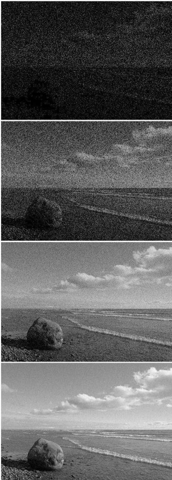
Modern electronic CCD pixels actually count individual photons of light. This is easily revealed in the dramatic short time exposure photos seen to the left, of a scene taken under very low light levels. The human retina is also an organic light imager that can detect individual photons of visible light.
