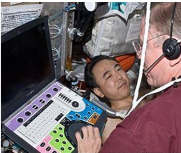
A next-generation ultrasound device for astronaut care and improved ISS research capabilities was delivered to ISS by STS-135, replacing a decade-old machine. The Ultrasound 2 is a commercial off-the-shelf system that was updated to meet space flight standards, and will be a key tool in research for long-duration human exploration. The ultrasound images sent back to Earth allow biomedical researchers to better understand and monitor changes in the human body during space flight. Astronaut Mike Fossum is using Ultrasound 2 to scan JAXA crewmember Satoshi Furukawa.
