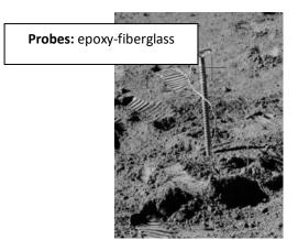
Figure B7 – Heat Flow Experiment
