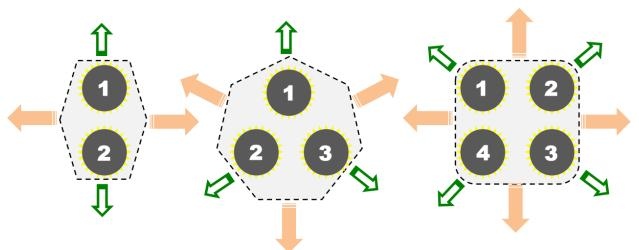
Figure 3: Diagram of multiple engine spacecraft ejecta paths – orange (solid) arrow denotes direction of maximum ejecta flux 'rooster tail' along plume reflection planes.
