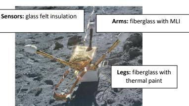
Figure B4 – Lunar Surface Magnetometer
