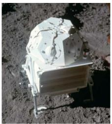
Figure B5 – Solar Wind Spectrometer
