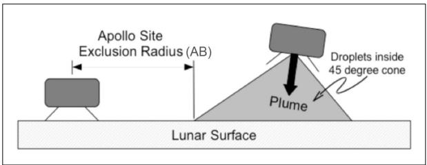
Figure 12: Illustration of plume droplet cone.
