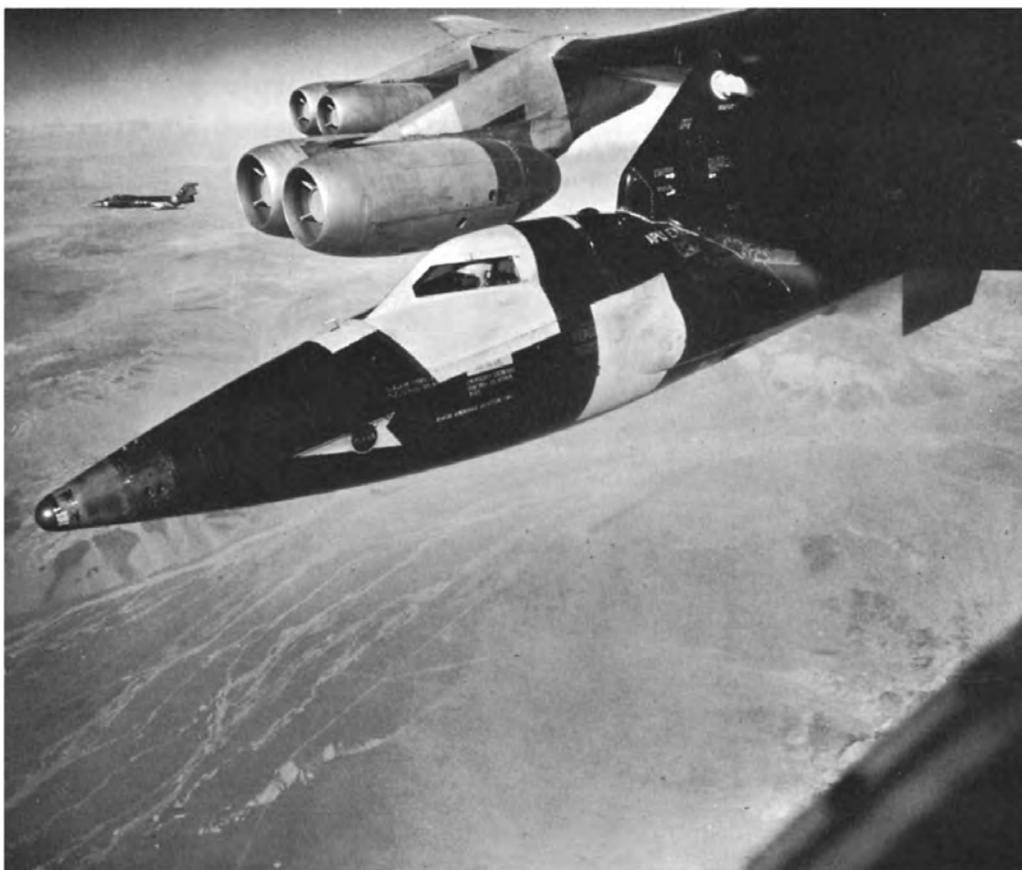
An X-15 is seen just prior to launch from a B-52 at 45 000 ft., 200 miles from home base. The X-15 pilot und B-52 launch-panel operator have completed their pre-launch check procedures. The chase plane in the distance is keeping a sharp eye on the X-15 during the checkout.
