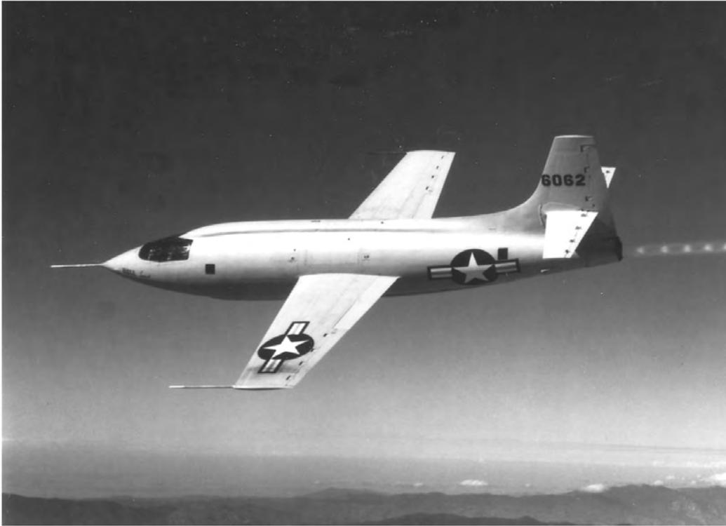
Noted predecessors of the X-15 in the cooperative research-airplane program of the Air Force, Navy, and NACA, dating from 1944, were the X-1 (above), which made the world's first supersonic flight, and the X-2 (below), which first flew to Mach 3.
