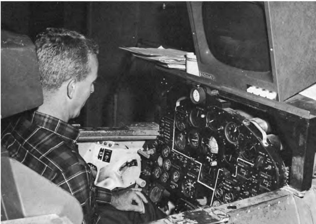
Before each 10-12-minute research mission, X-15 pilots train as long as 10 hours in the electronic simulator at Edwards AF Base. Chief Research Pilot Walker is sitting in its cockpit here. The simulator duplicates the X-15's cockpit, instruments, and control system, including hydraulics and dummy control surfaces, and is nearly as long as the aircraft itself.
