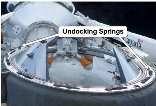
Figure 5: Entire view of the undocking springs on the space shuttle's ODS
