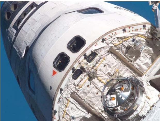
Figure 1: Space shuttle payload doors have opened, revealing the Orbital Docking System.
