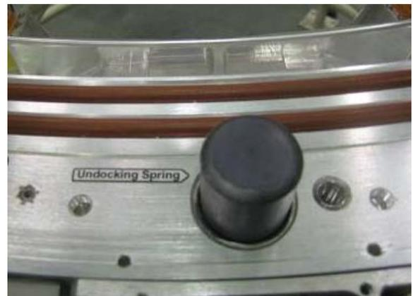
Figure 6: Close-up view of an undocking spring on the ODS training unit
