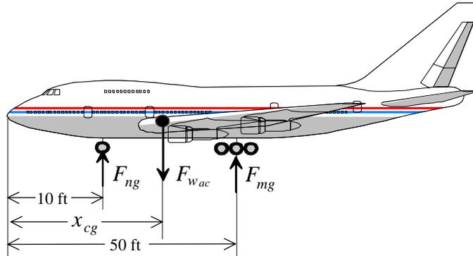
Figure 2 Measuring Weight and Center of Gravity
