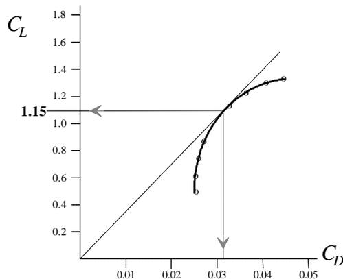
**Step 5:** Put the  $C_L$  found in step 4 into Equation 8.3 and solve for the best endurance airspeed.
