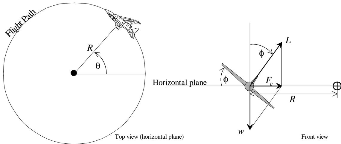
Figure 4 An Airplane in a Level Turn
