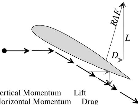
Figure 4.9 Resultant Aerodynamic Force
