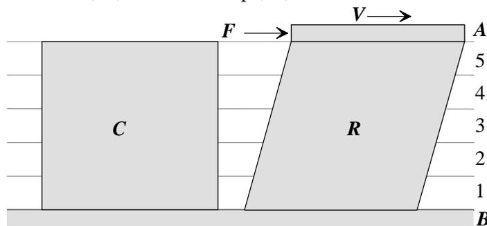
Figure 1 Viscous Friction
