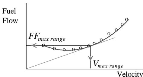
Figure 8.8 Determining Maximum Range Airspeed and Fuel Flow
