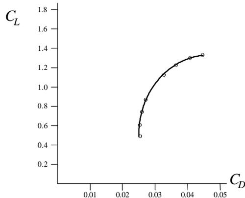
**Step 3:** Draw a line from the origin tangent to the curve.
