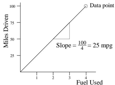
Figure 8.1 Ratio of Miles Driven vs. Fuel Used
