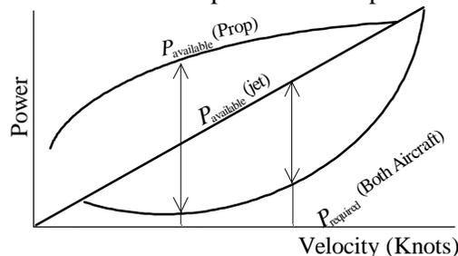
Figure 7.9 Maximum Rate of Climb, Prop and Jet
