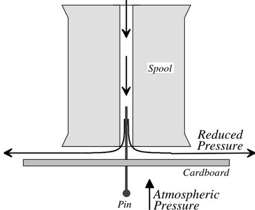
A jet of air moves horizontally from the hole at the bottom and spreads out over the surface of the cardboard. If air is blown through with sufficient speed, the outward movement of the air at the
