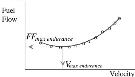
Figure 8.9 Determining Maximum Endurance Airspeed and Fuel Flow
