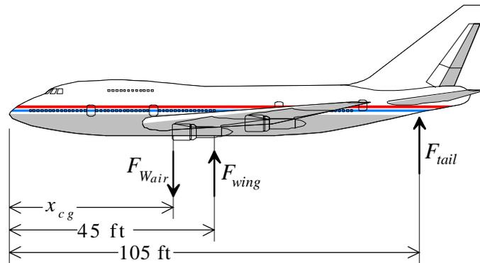
Figure 3 Level Flight Forces and Moments
