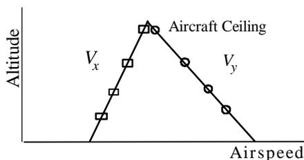
Figure 7.14 Variation of  $V_x$  and  $V_y$  with Altitude
