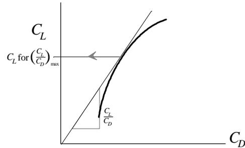
Figure 8.5 Determining Tangent
