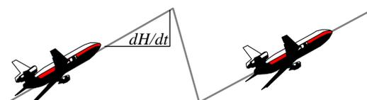
Figure 7.11 Sawtooth Climb Technique
