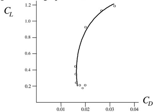
**Step 3:** Draw a tangent line from the origin to the curve.
