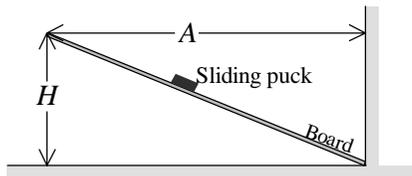
Figure 4.2 Coefficient of Friction,  $C_f = \tan C = \frac{H}{A}$
