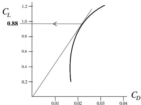
**Step 5:** For this value of  $C_L$ , use Equation 8.3 to determine the velocity for an aircraft which weighs 9000 pounds.
