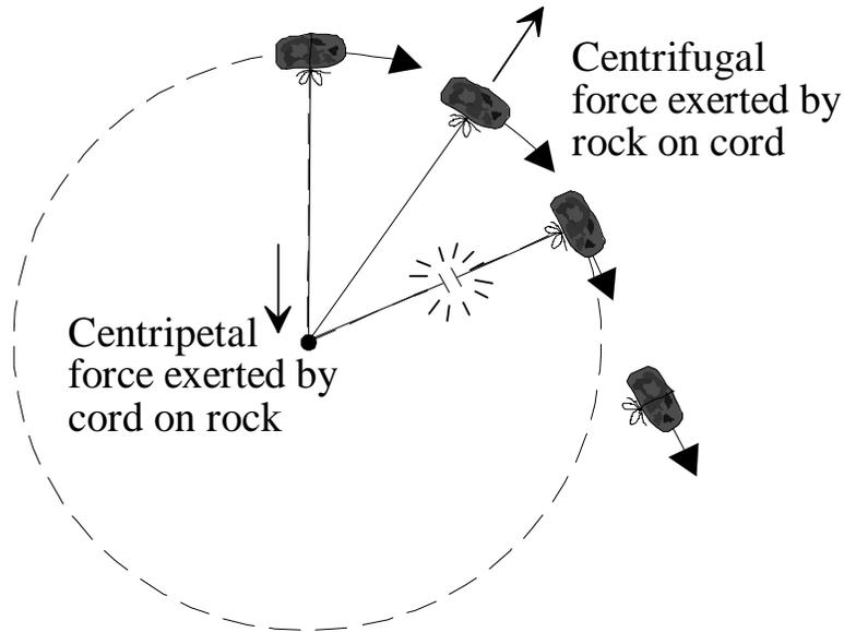
Figure 2 Centripetal and Centrifugal Forces
