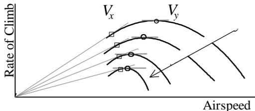
Figure 7.13 Climb Data as a Function of Altitude
