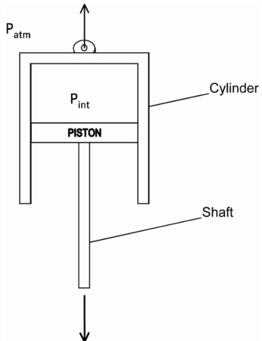
Figure 3: Cross-sectional force diagram of one ARED piston/cylinder assembly
