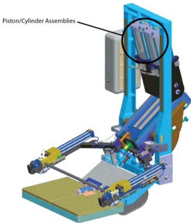
Figure 2: A model of ARED showing the piston/cylinder assemblies
