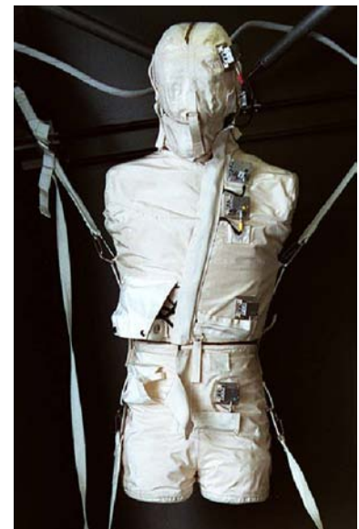
NASA uses an anatomical model of a human torso and head that contains more than 300 radiation sensors.
