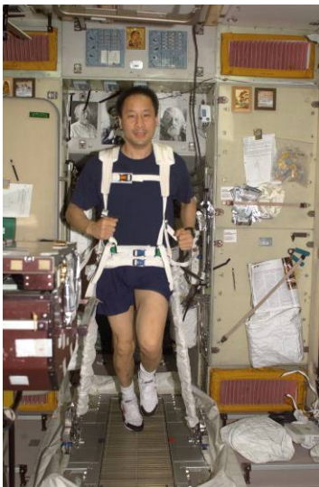
Figure 1: Astronaut Edward T. Lu exercises on the Treadmill Vibration Isolation System (TVIS) on the International Space Station (ISS).
