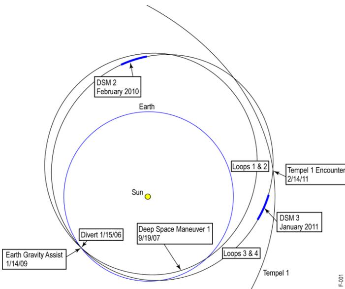
The trajectory of the Stardust-NExT mission consists of four loops of the sun in two separate orbits. Loops 1 and 2 represent the orbit the spacecraft bus was left in after the sample return on Jan. 15, 2006. The Earth gravity assist on Jan. 14, 2009 placed the spacecraft in the final heliocentric orbit (Loops 3 and 4) intercepting Tempel 1 on Feb. 14, 2011 (39 days after the comet's perihelion).
