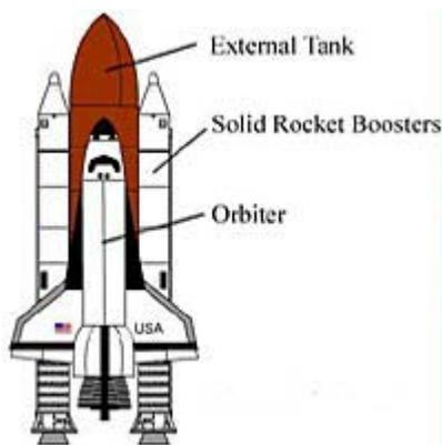
Figure 1: Main components of the space shuttle
