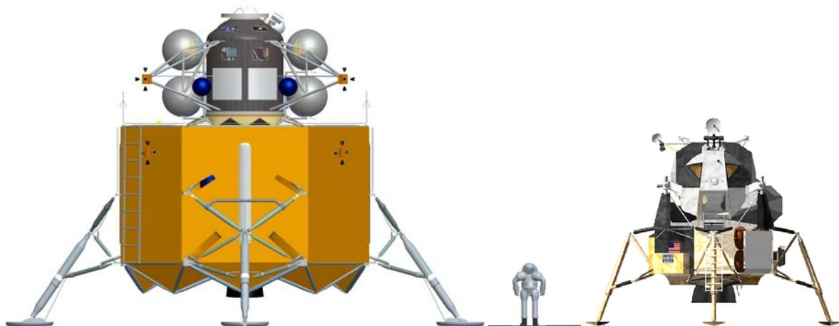
Figure 1: Comparison of the new lunar lander, Altair, (left) (NASA concept) and the Apollo LEM (not to scale)
