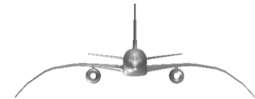
Drooped-Wing Vehicle Concept 5.3% Drag Reduction
