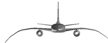
Squashed-Fuselage Drooped-Wing Vehicle Concept 15% Drag Reduction
