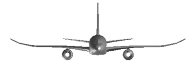
Inflected-Wing Vehicle Concept 3.5% Drag Reduction
