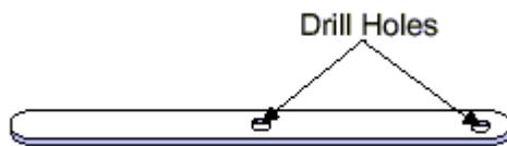
3. Each student will need four drilled sticks and four brass paper fasteners. Note: dampening the sticks before drilling can reduce cracking the wood.
