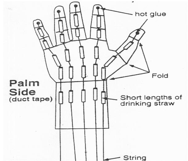
Robots are often used to assist humans. In this activity, students will create an end effector designed to replicate the human hand.
