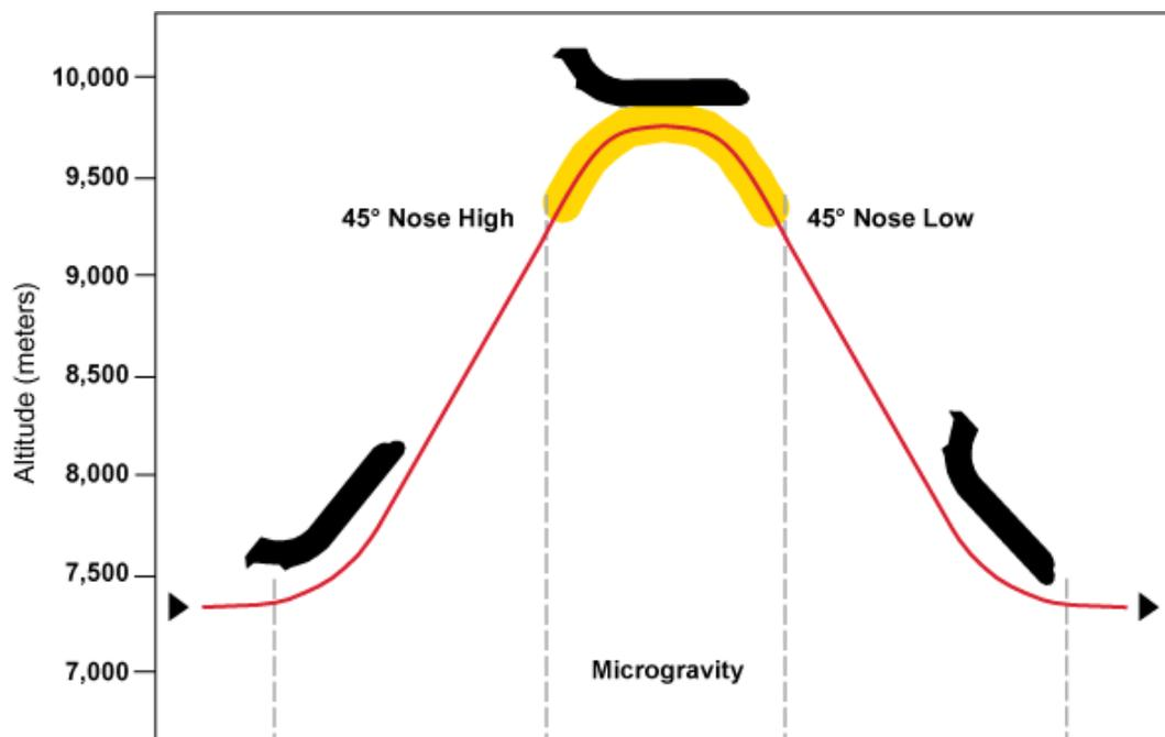
Figure 3: A typical microgravity maneuver. (not to scale)
