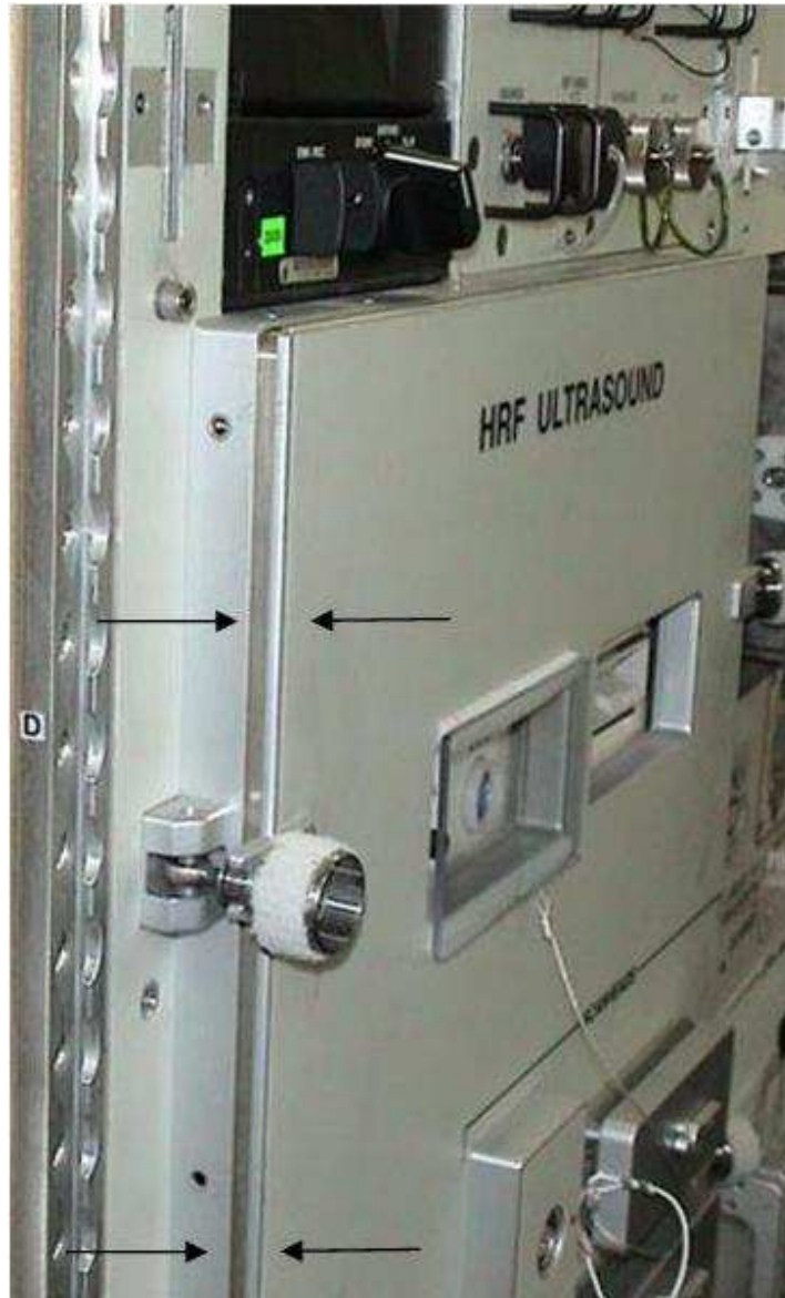
Figure 7. - Illustration of Symmetrical Gap When Reinstalling HRF Ultrasound Front Panel.
