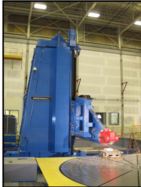
Ares Vertical Milling Machine during initial “circle, diamond, square” acceptance test in 4705
