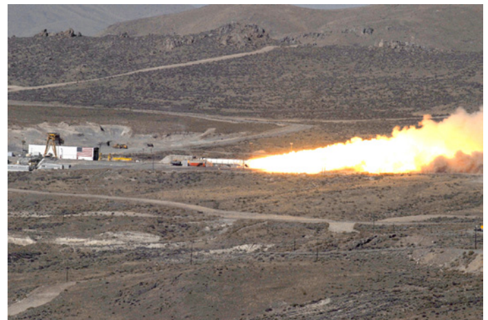
A space shuttle reusable solid rocket motor billows smoke and fire during a two-minute static test Nov. 1, 2007, at a Utah test facility. Image Credit: ATK
