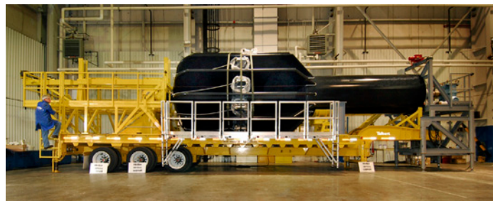
ATK technicians inspect the new Ares I first stage forward casting core for the five-segment booster after delivery to ATK Space Systems in March 2008.
