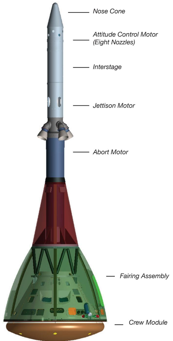
pull the crew safely away from the Ares I stack in an emergency. It will use four exposed, reversed flow nozzles to provide the initial abort impulse. An attitude control motor composed of eight nozzles will orient the abort vehicle as it pulls away from the launch vehicle.
