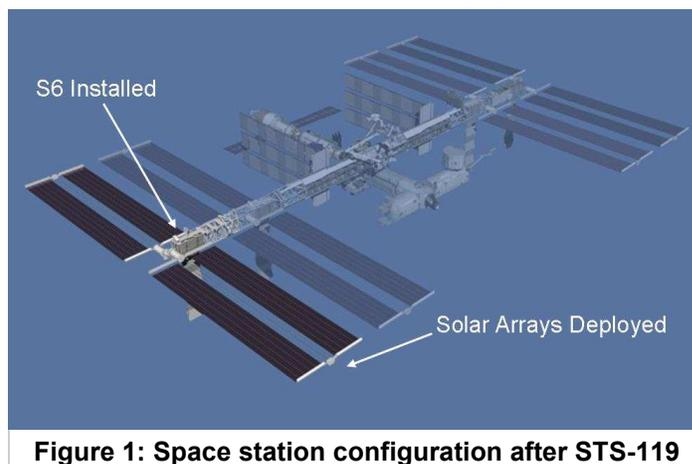
**Figure 1: Space station configuration after STS-119**
