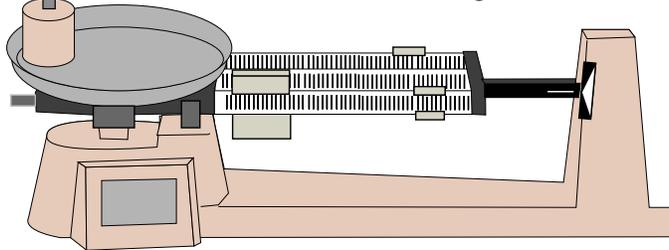
Adjusting the slide weights provides a measure of the force being exerted on the rocket.
