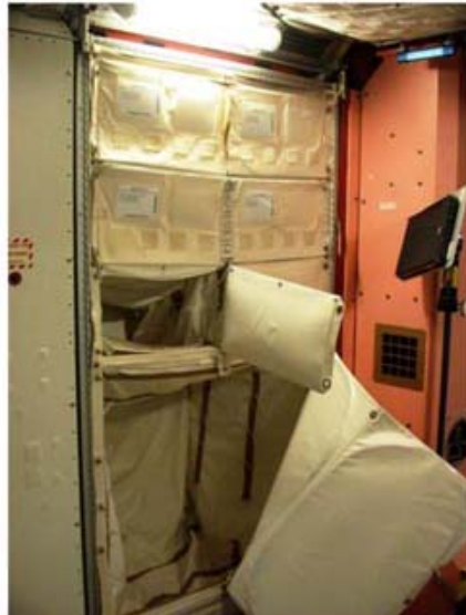
Figure 16. - Open ZSR Doors.
