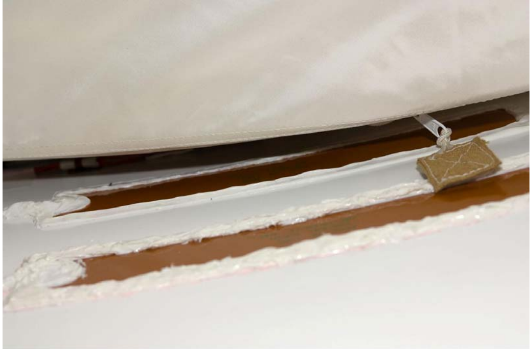
Figure 13.- ZSR Zipper and Cloth Tab improperly contacting JEM shell heater.
