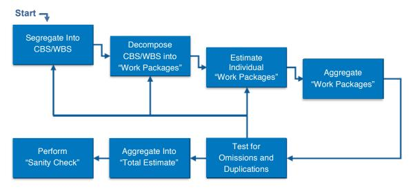
Figure 8. Method for Developing Engineering Build-Up Estimate
