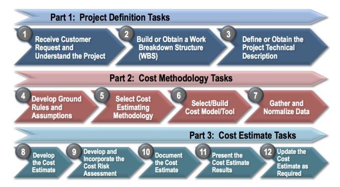
**Figure 2. The NASA Cost Estimating Process**
