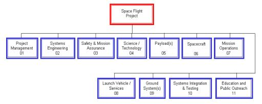
Figure 4. Standard Flight Project Level 2 Work Breakdown Structure<sup>7</sup>
