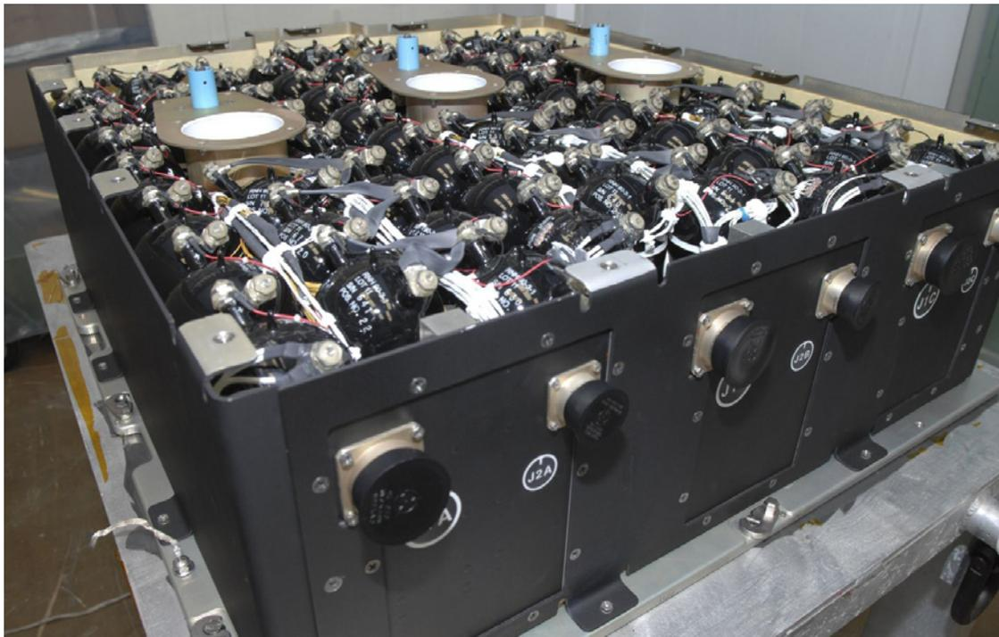
*Battery Module Assembly with lid removed, showing the cells and power isolation switches.*
