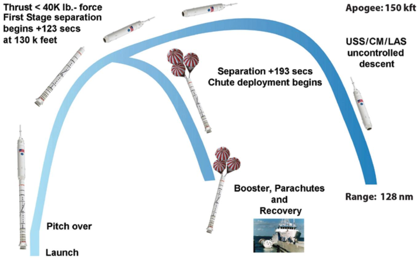
The flight of Ares I-X is designed to simulate the first two minutes of Ares I flight. A broad range of performance data will be relayed to the ground. The solid rocket motor will separate and will be recovered at sea for later inspection. The simulated upper stage and Orion’s crew module and launch abort system will not be recovered.
