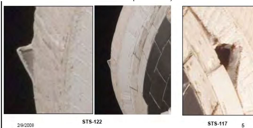
Figure 2 - R OMS Pod Blanket pulled back
