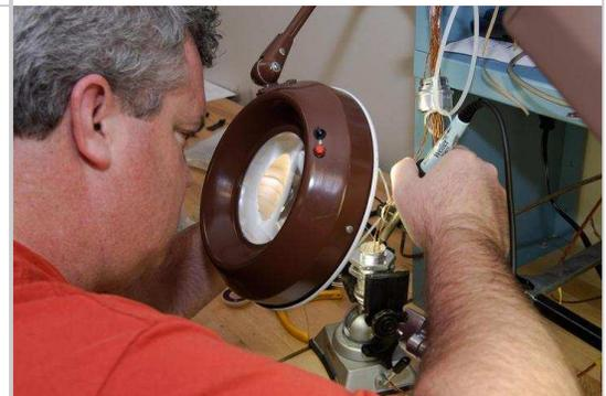
At a lab at Kennedy, Bob Arp, United Launch Alliance technician, solders a pin to the socket of the replacement feed-through connector
