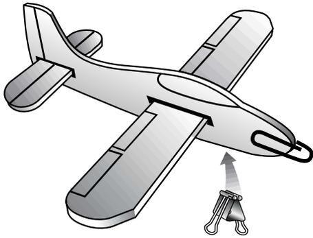
1. The model glider's weight must be balanced or distributed properly before it will fly. To demonstrate this, ask a student to launch a glider before adding weight and balance. Have students describe the flight characteristics.
