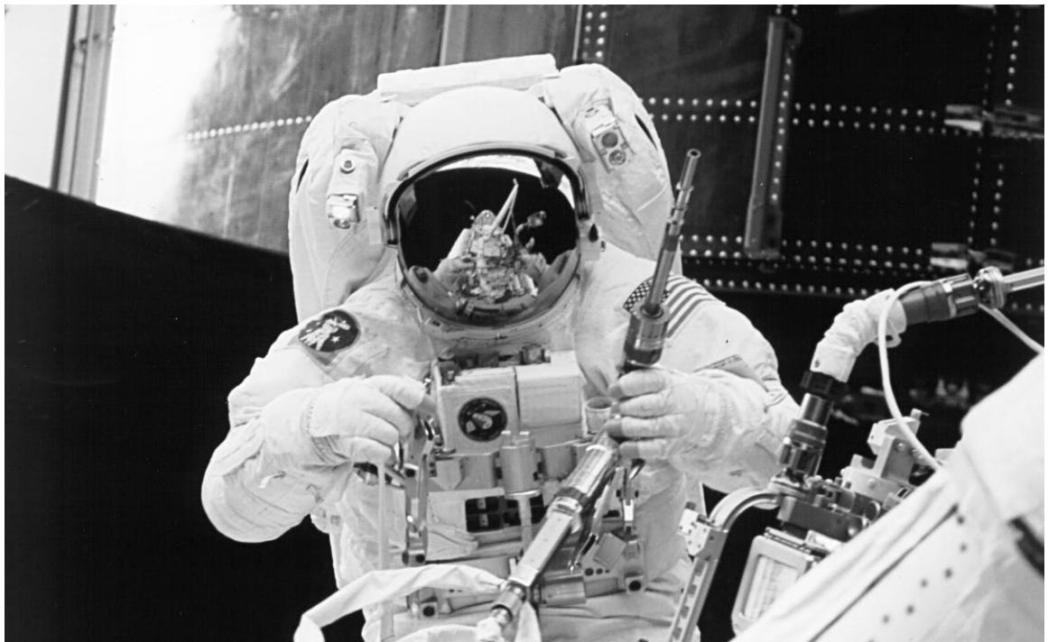
STS-82 Astronaut Steven L. Smith holds a power ratchet tool as he prepares to replace some of the instruments on the Hubble Space Telescope.
