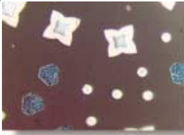
Results from a microgravity experiment in sintering have led a researcher to discover that gas plays more of a role in the process than was believed. Here large pores or holes formed by gases are shown unexpectedly coalescing in the experiment sample.
