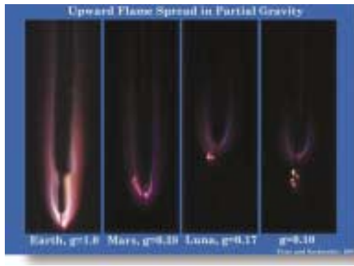
A fire on the Moon or Mars behaves differently than it would on Earth because of differences in the amounts of gravitational force on these planets. Upward flame spreading over paper samples at four different gravity levels is shown in these images. Varying gravity levels were obtained using NASA's KC-135 aircraft as it maneuvered through a parabolic flight path. As gravity is reduced, the buoyant, upward motion of air is slowed and the flames become shorter and spread more slowly.
