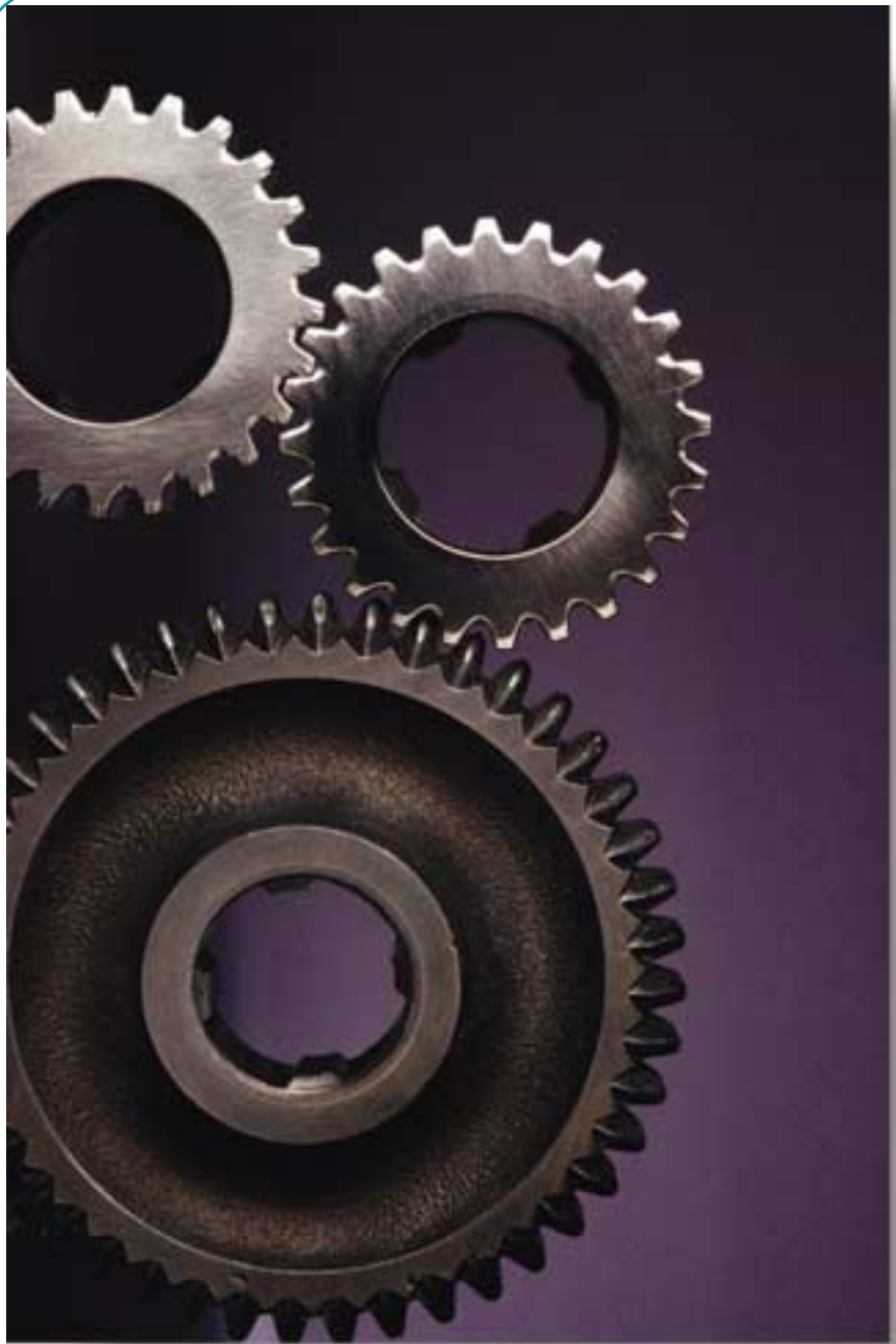
Items too small and precise for machining are produced by sintering. Microgravity research is contributing to a better understanding of this process on the ground and may lead to improved manufacturing of sintered products.
