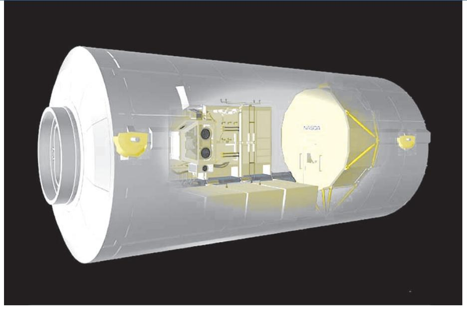
*The Centrifuge Accommodation Module will host gravitational biology investigations on board the International Space Station. The 2.5-m-diameter centrifuge allows for experimentation at various g levels.*
