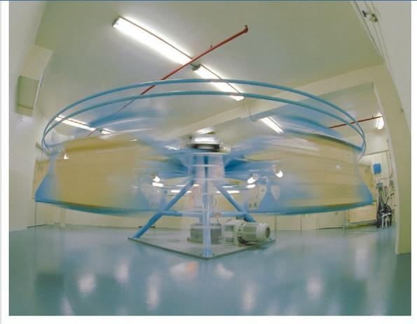
*The 24-foot-diameter centrifuge (spinning) is one of the Center for Gravitational Biology Research facilities.*
