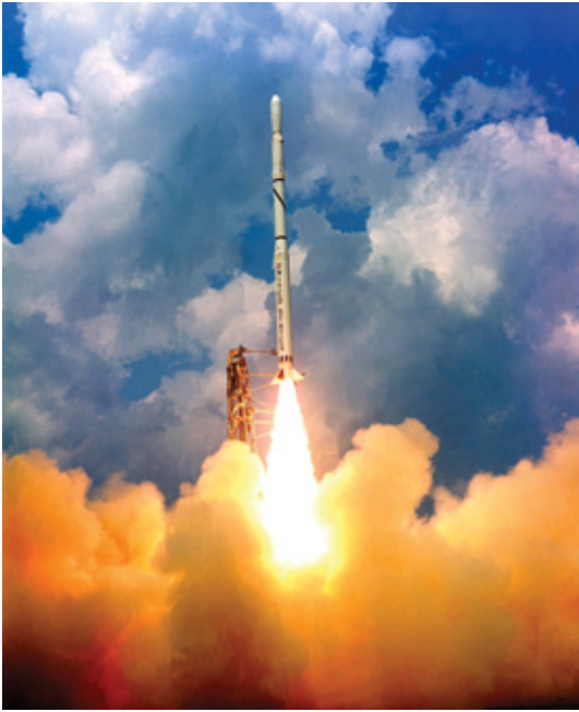
Four-stage, solid propellant Scout rocket.
