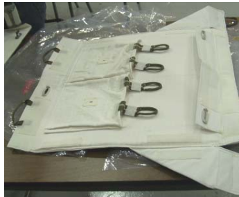
Figure 1.– Lid and hinge flaps with quarter turn fastener openings
