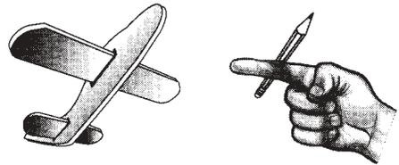
Hint: The weight of the model glider must be balanced before it will fly successfully. To determine the “Center of Gravity” of the glider, the model can be balanced much like a pencil on their finger (diagram).
