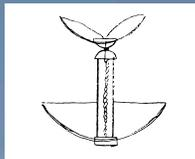
The Flying Toy: A small toy "helicopter"—made of wood with two twisted rubber bands to turn a small propeller—that the Wright brothers played with as small boys.
