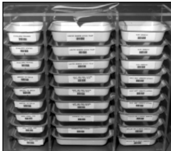
International Space Station frozen food storage: Food will be stowed in pullout drawers, which allow complete viewing of drawer contents. Lipped edges on the food package interface with the storage container, oven, and serving tray.
