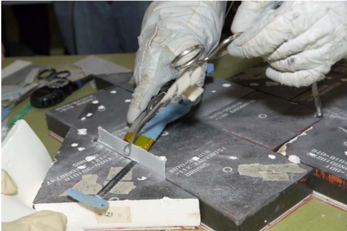
Figure 12 Stbd Gap Filler Cutting
