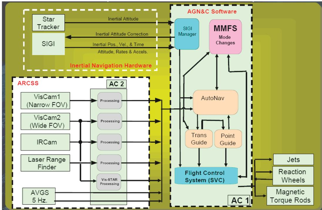
Figure 5.1-1. OE AGN&C System Block Diagram (from ref.1)
