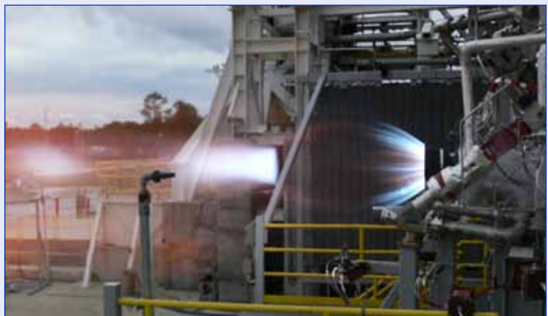
Blue Origin successfully test fires its BE-3 high-performance liquid hydrogen engine thrust chamber at NASA's Stennis Space Center. (Image credit: Blue Origin)
