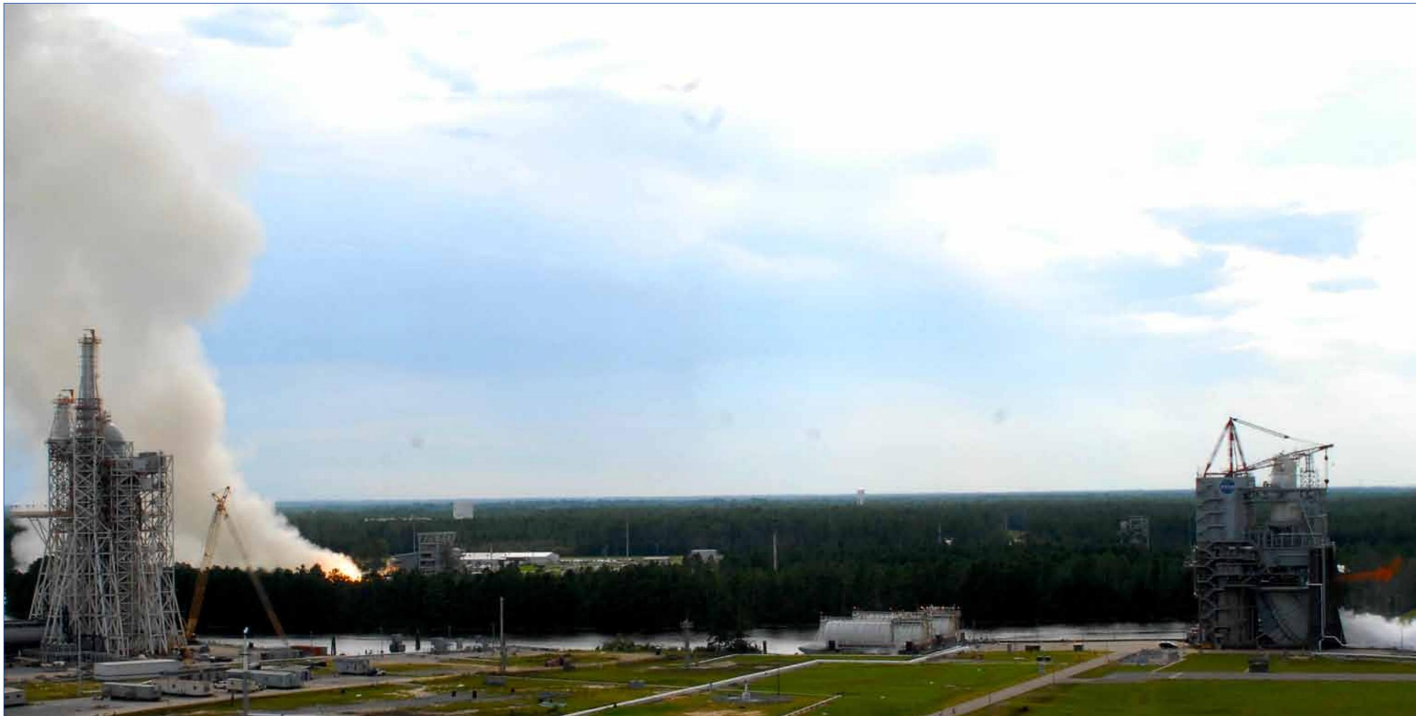
Two large-engine tests were conducted simultaneously for the first time at Stennis Space Center on Aug. 16. A plume on the left indicates a test on the facility's E-1 Test Stand. On the right, a finger of fire indicates a test
