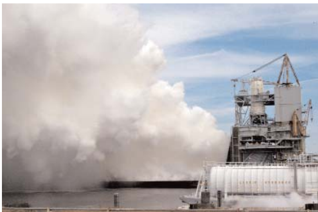
A test conducted Feb. 12, 2007, on Stennis Space Center's A-2 Test Stand helps engineers certify a seal inside the high-pressure oxidizer turbo pump of a space shuttle main engine. The test was part of a critical series to help keep the space shuttle's flight schedule on track.
