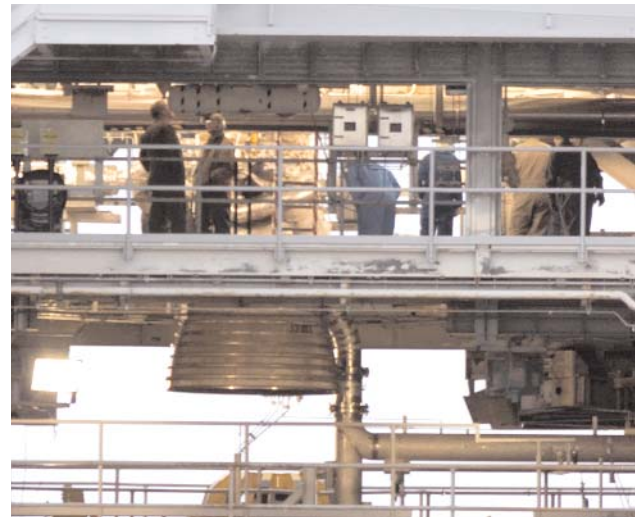
MILESTONE MOMENT – Dwarfed by the J-2X powerpack installed on the A-1 Test Stand's Level 5, Stennis Space Center workers evaluate the status of the test article and its Powerpack 1A following a chill test Dec. 18.
