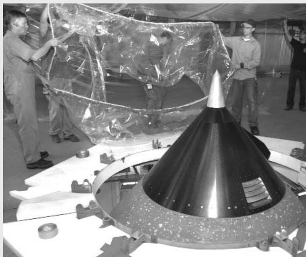
On an upper level of high bay 1 of Kennedy Space Center's Vehicle Assembly Building, technicians move protective material toward the nose cone of Atlantis' external tank.
