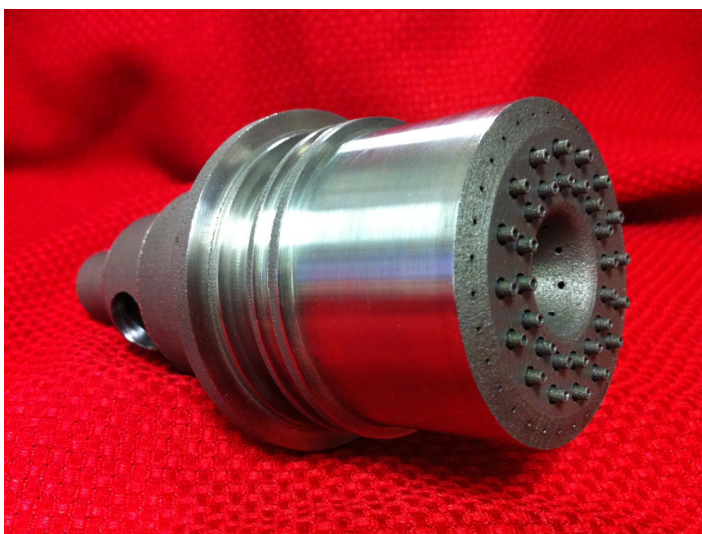
Materials engineers made this one-piece rocket engine injector in just 40 hours in a sophisticated 3-D printing machine at Marshall's Advanced Manufacturing Facility. It takes much longer to manufacture the same part by welding multiple parts. (NASA/MSFC/Sandra Greene)
