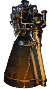
The Fastrac engine is a new, 60,000-pound-thrust engine that will be used for the first powered flight of NASA's X-34 technology demonstrator. The first engine developed in-house by engineers at NASA's Marshall Space Flight Center in Huntsville, Ala., Fastrac went from the drawing board to the test stand for full-engine, hot-fire testing in less than three years—a much faster than usual design cycle for rocket engines.
