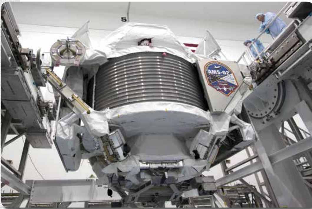
In the Space Station Processing Facility, the Alpha Magnetic Spectrometer-2 (AMS) is positioned to provide better access for work to be performed on its avionics box. AMS was delivered to the International Space Station aboard space shuttle Endeavour's final flight, the STS-134 mission.
