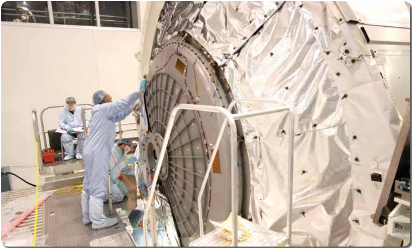
In the Space Station Processing Facility, technicians installed insulating blankets to the hatch of the Permanent Multipurpose Module (PMM) to protect it from the harsh environment and temperatures of space. The PMM was delivered to the International Space Station aboard space shuttle Discovery's final flight, the STS-133 mission.
