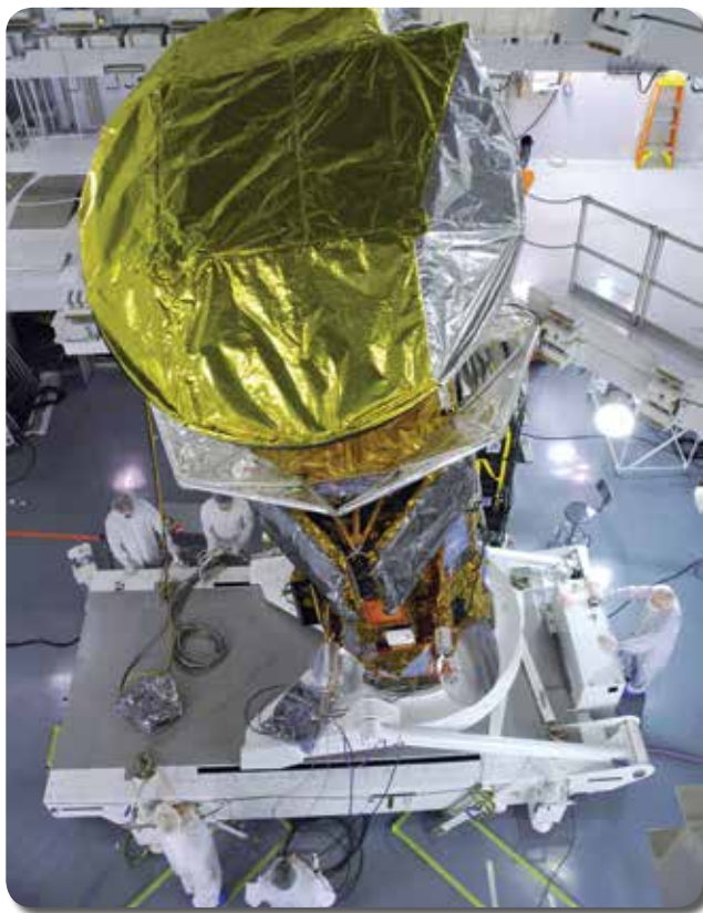
In Space Systems International's Payload Processing Facility at Vandenberg Air Force Base in California, technicians rotate the Aquarius/SAC-D spacecraft into a vertical position for testing on April 12, 2011.
