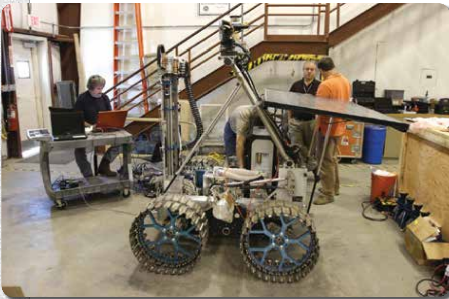
The NASA payload is installed on the prototype rover Artemis Jr. for the Regolith and Environment Science and Oxygen and Lunar Volatile Extraction, or RESOLVE, project in a test facility behind the Operations and Checkout Building.
