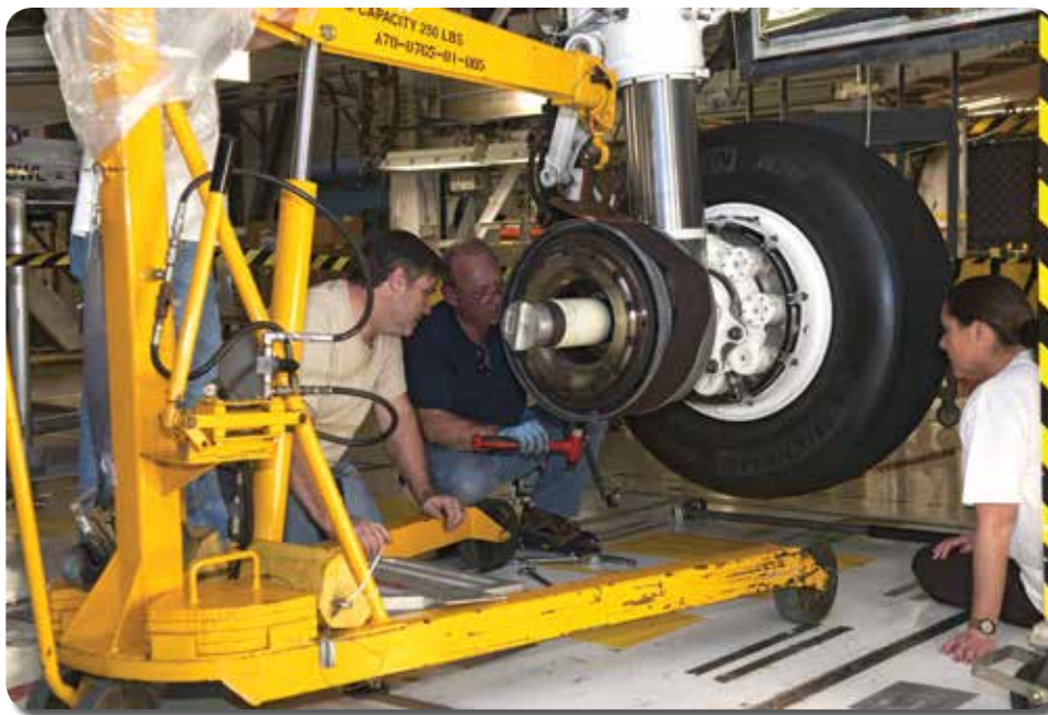
In Orbiter Processing Facility-2, United Space Alliance mid-body shop mechanical technicians remove the main landing gear brakes on space shuttle Endeavour to prepare for the STS-134 mission. The shuttle's tires were replaced following each flight, and the brakes were replaced after every eighth flight.
