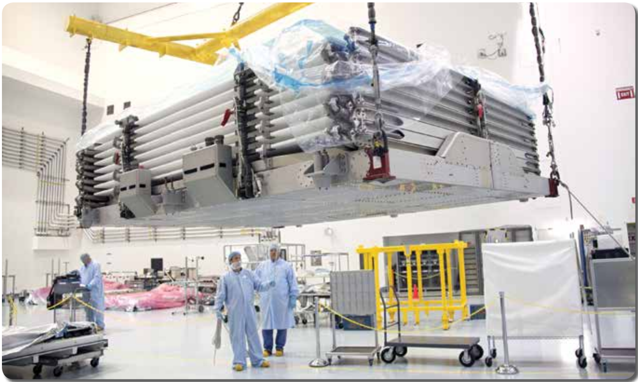
Workers in the Space Station Processing Facility monitor the progress of the Heat Rejection Subsystem as it was transported by an overhead crane toward the Express Logistics Carrier-4, or ELC-4. Space shuttle Discovery delivered the ELC-4, filled with external payloads and experiments, to the International Space Station on its final flight, the STS-133 mission.
