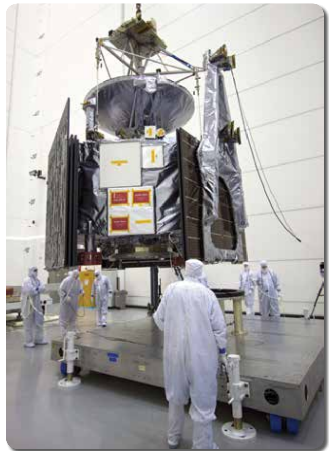
At Astrotech's Hazardous Processing Facility in Titusville, Fla., technicians using an overhead crane lower NASA's Juno spacecraft to a fueling stand where the spacecraft was loaded with the propellant necessary for orbit maneuvers and the attitude control system on June 27, 2011.
