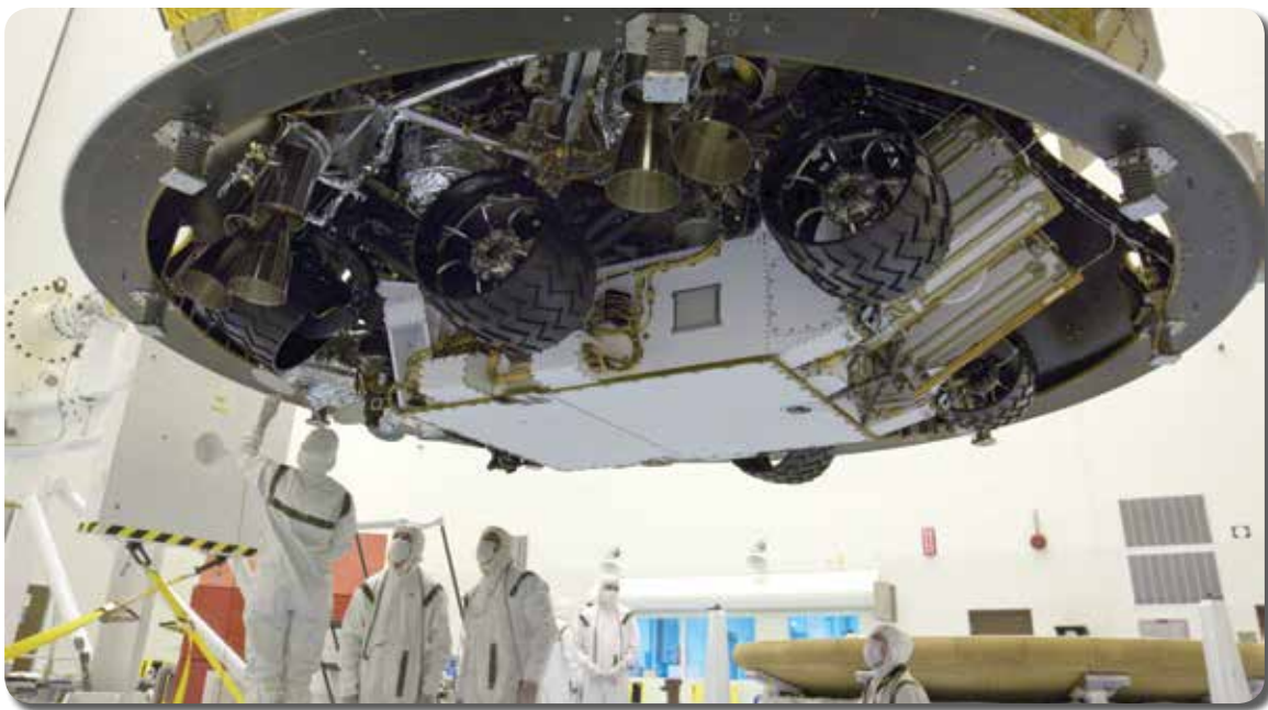
In the Payload Hazardous Servicing Facility at NASA's Kennedy Space Center in Florida, technicians work beneath NASA's Mars Science Laboratory mission aeroshell, containing the compact car-sized rover Curiosity, which was mated to the cruise stage, on Oct. 11, 2011.
