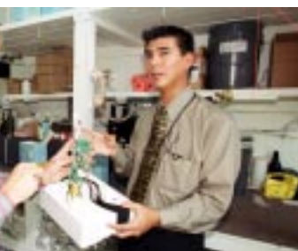
supervisor of meteorology and Dave Chapman, upper air systems controller, radiosonde operates. A radiosonde is carried through the atmosphere and routinely provides data to an altitude of 20 miles.
