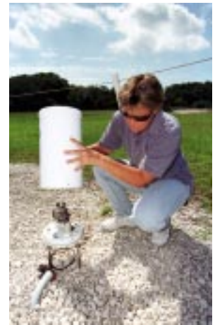
Stacie Price inspects a tipping rain gauge for obstruction.
