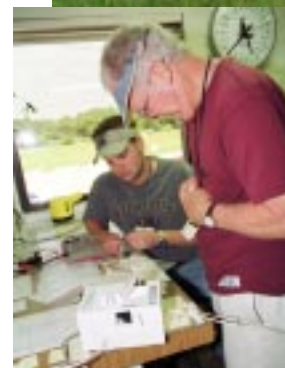
Above, Computer Sciences Raytheon meteorological data specialists Stephen Ezell (foreground) and Mike Boyer preparing a new GPS-tracked radiosonde for flight. At top, the two tie the radiosonde to a parachute and a helium-filled weather balloon just prior to release.
