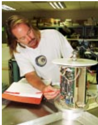
Bill Ulbircht makes repairs to a lightning warning sensor.
