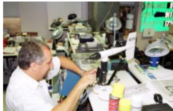
Meteorological electronic specialist Alan Petit repairs an anemometer. Anemometers are sensors that provide wind speed and direction.
