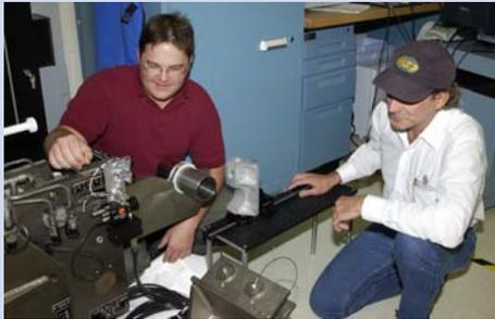
Dr. Chris Immer and Dr. John Lane of Dynacs discuss digital image processing techniques to precisely measure relative positions of the Payload Ground Handling Mechanism (PGHM), which loads cargo into the Orbiter Payload Bay.
