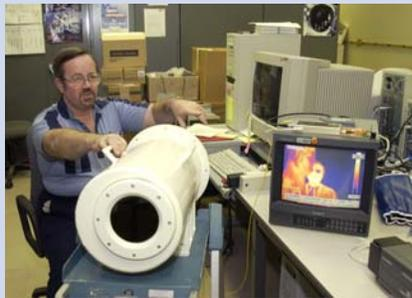
Carl Hallberg of Dynacs demonstrates the new Infrared Hydrogen Fire Detection Camera.
