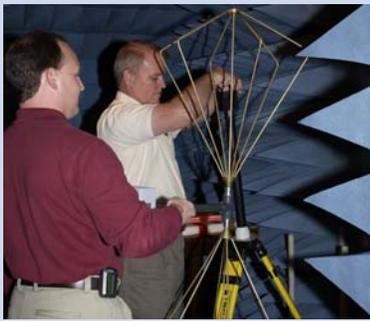
Dynacs' Tony Eckhoff and Mike Blalock set up instrumentation prior to testing in a chamber designed to detect electromagnetic interference.
