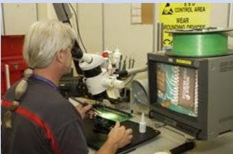
Jim Henderson of Dynacs replaces a miniature surface mount component on a circuit board.
