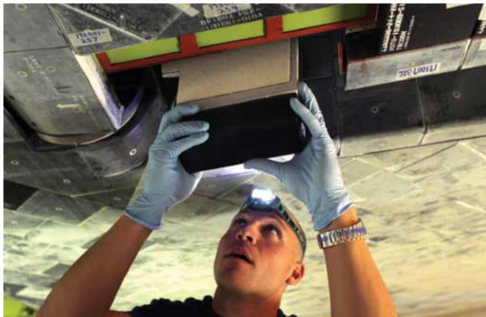
A United Space Alliance technician removes and replaces a hub tile on space shuttle Discovery before its STS-119 mission to deliver the S6 truss segment to the International Space Station.
