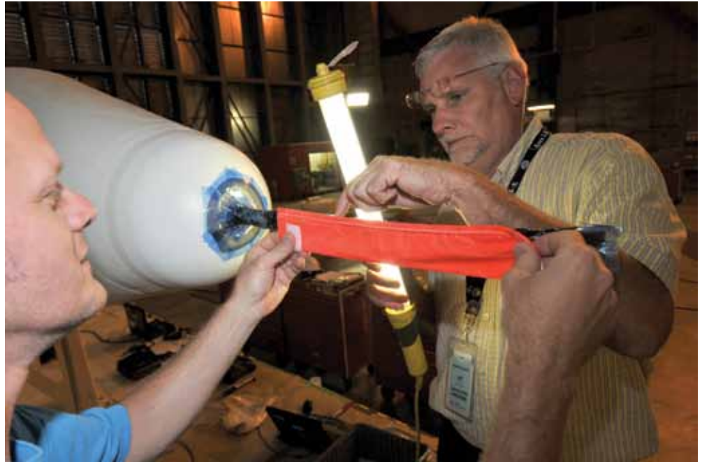
Inside Kennedy Space Center's Vehicle Assembly Building, or VAB, David Rowell, left, a NASA Prototype Laboratory technician, and Henry May, with Kennedy's Constellation Transportation Planning Office, perform a fit check on a cover for the tip of the Ares I-X probe.
