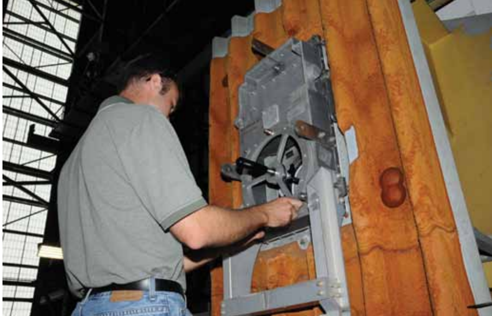
Inside Kennedy Space Center's Vehicle Assembly Building, or VAB, NASA Lead Engineer for the Prototype Development Laboratory Adam Dokos performs a fit check of the External Tank Hydrogen Leak Anomaly Measurement Tool on a mock-up of the fuel tank's umbilical plate for the STS-127 mission.
