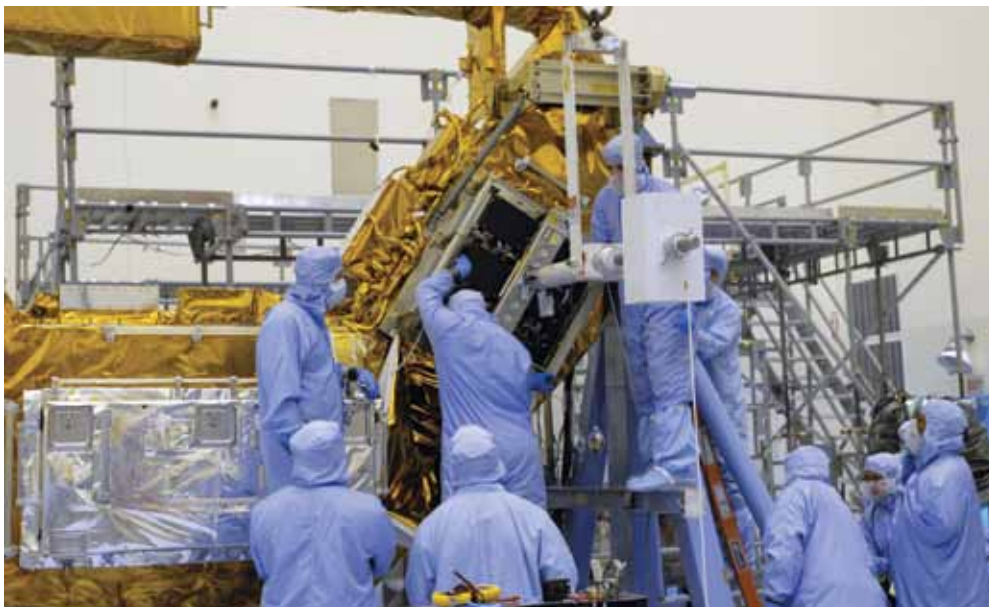
In the Payload Hazardous Servicing Facility at Kennedy Space Center in Florida, technicians check the Multi-Use Lightweight Equipment Carrier where the Science Instrument Command and Data Handling Unit was housed for the fifth and final shuttle servicing mission to NASA's Hubble Space Telescope.
