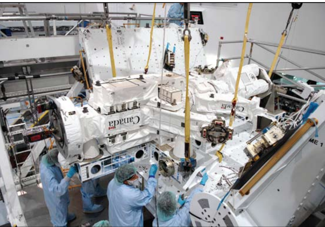
Technicians adjust the Canadian Space Agency's special purpose dexterous manipulator, known as Dextre, into position on a pallet inside the Space Station Processing Facility.
