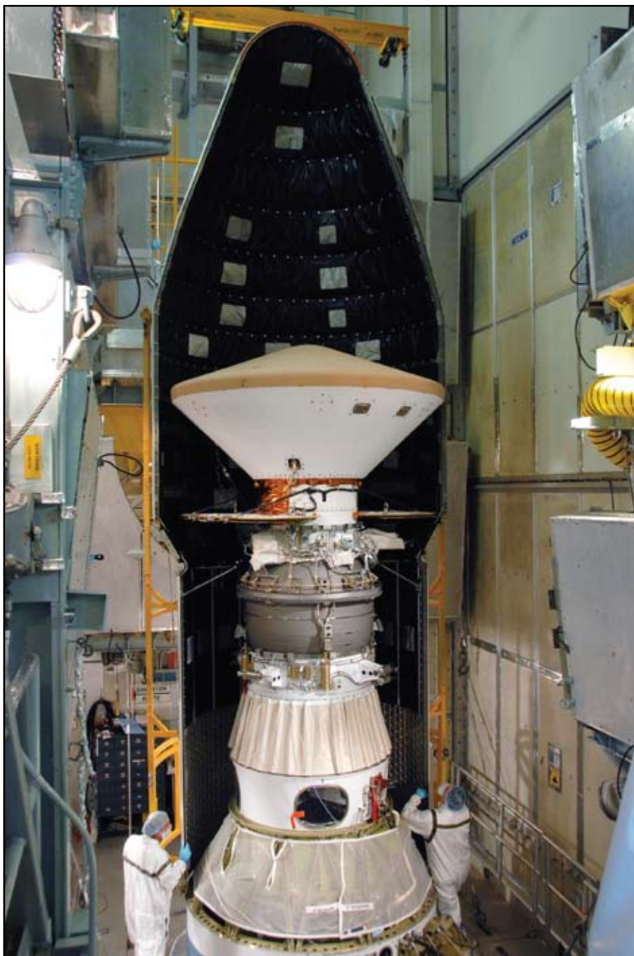
On Launch Pad 17-A at Cape Canaveral Air Force Station, the first half of the fairing is moved into place around the Phoenix Mars Lander for installation.
